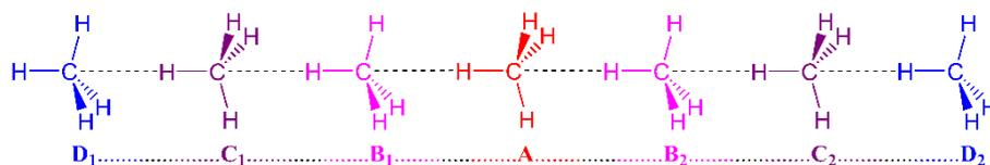
**Figure 1.** Model system composed of 7 linearly arranged methane molecules (middle molecule A plus three surrounding layers B, C and D)
